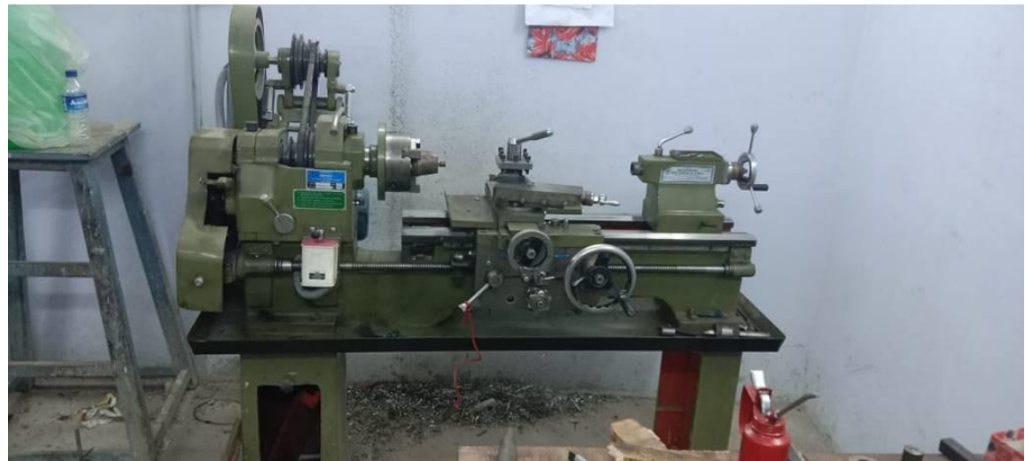
Conventional Turning machine holding capacity of Dia 200mm
