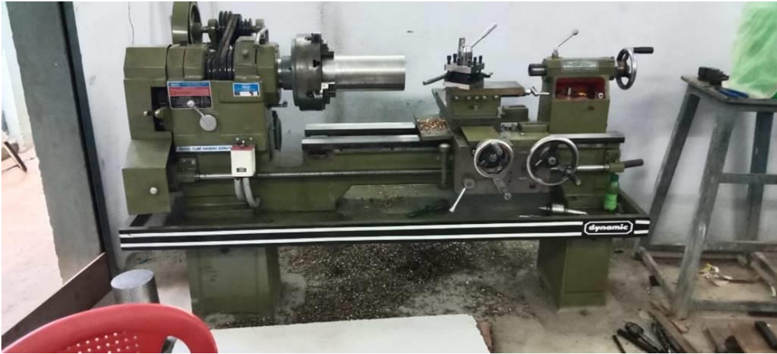
Conventional Turning machine holding capacity of Dia 600mm
