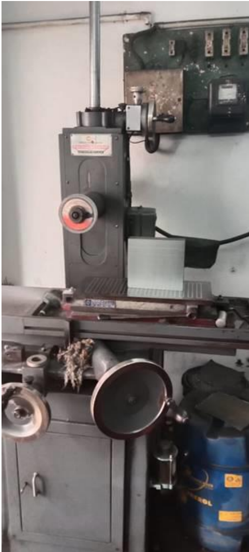
New Surface Grinding Machine Of Guru Arjan Brand, Bed Size 450x250x300mm
